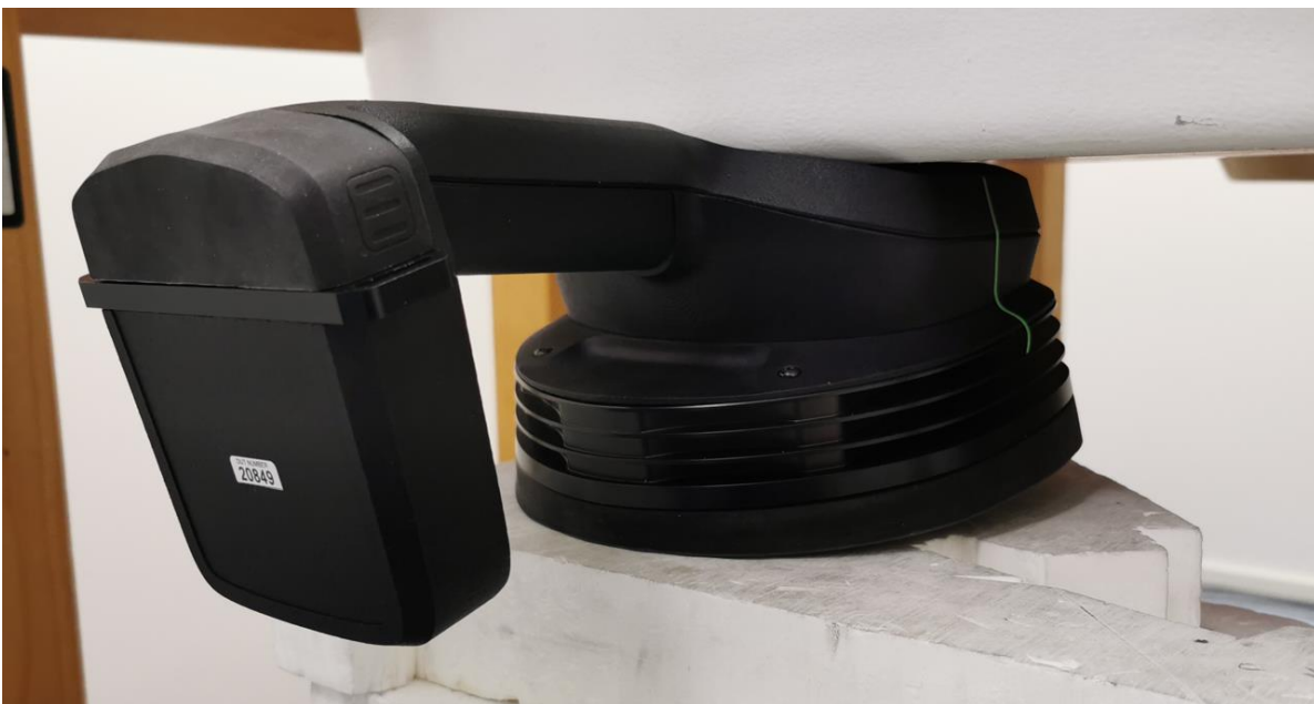
Figure 7 Back side of the DUT against the phantom, 0mm separation distance
