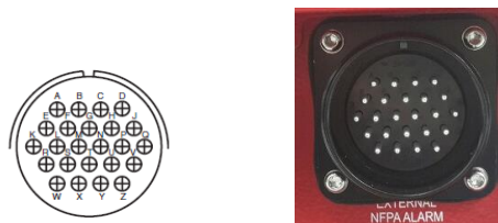
Figure 2 - 4 EXTERNAL NFPA ALARM Port
