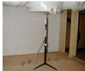
Figure 10-2 System Verification Setup Photo
