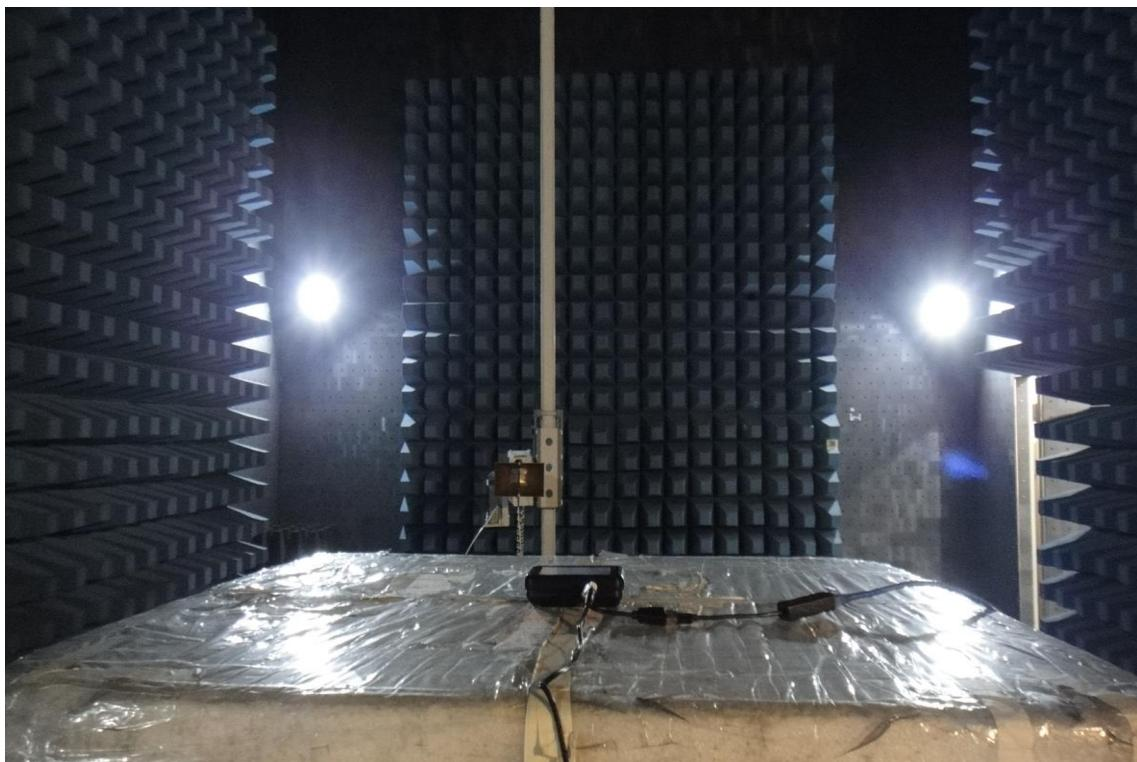
**Conducted Emission Set Up Photo**
