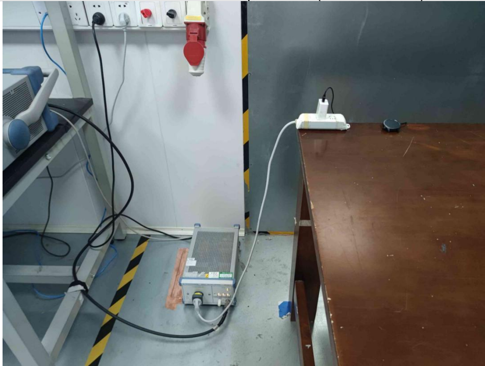
Conducted emissions at AC power line (150kHz-30MHz)
