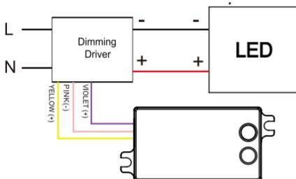
ANT-9-BLE-GE Wiring by AC/DC Adapter with dimming ballast or led driver.
