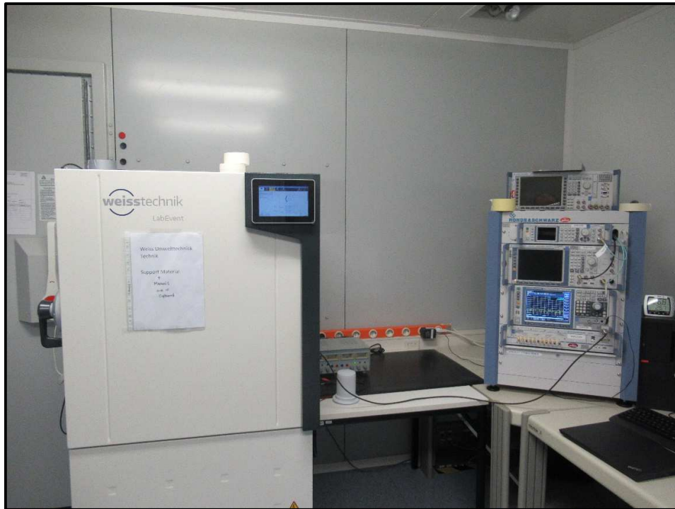
Photo 7: Conducted Test Setup
