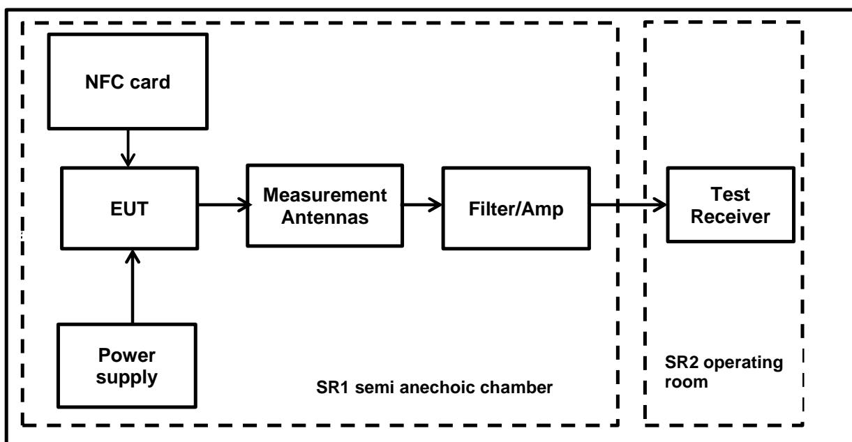
**Transmitter Radiated Emissions (continued)****Results: AC-DC Power supply / NFC 13.56 MHz**
