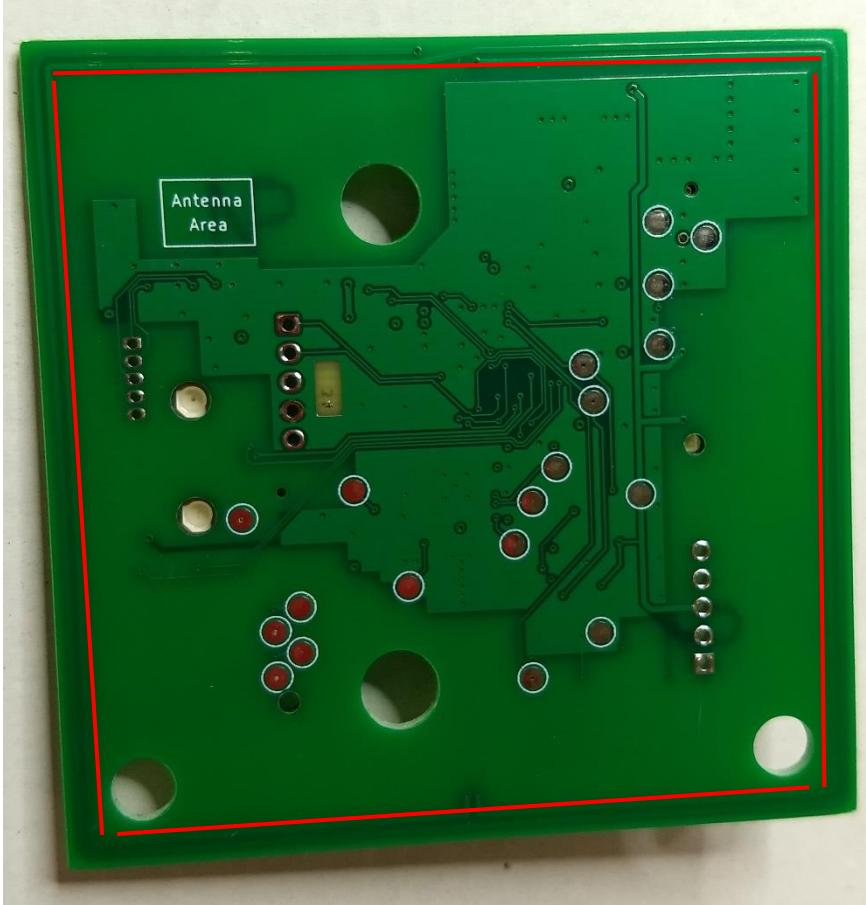
Antenna around the edge of the PCB see red lines
