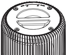
3. Before using, remove the filter from the plastic packaging and place the filter back into the device.
