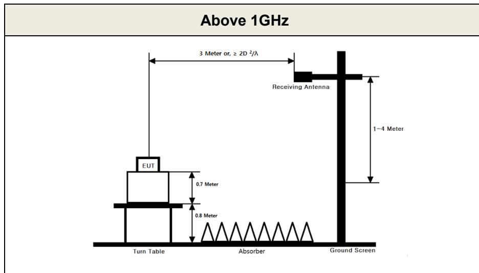
These measurements were performed at 3 m test site. The equipment under test is placed on a non-conductive table 1.5-meters above a turntable which is flush with the ground plane and 3 meters from the receive antenna. For measurements above 1GHz absorbers are placed on the floor between the turn table and the antenna mast in such a way so as to maximize the reduction of reflections. For measurements below 1 GHz, the absorbers are removed.
