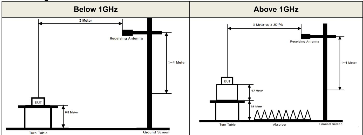
These measurements were performed at 3 test site. The equipment under test is placed on a non-conductive table 1.5-meters above a turntable which is flush with the ground plane and 3 meters(for below 1GHz: 0.8-m) from the receive antenna. For measurements above 1GHz absorbers are placed on the floor between the turn table and the antenna mast in such a way so as to maximize the reduction of reflections. For measurements below 1 GHz, the absorbers are removed.
