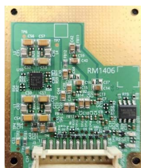
<Top> <Bottom> RM14-06A Radar Module (Side position)
