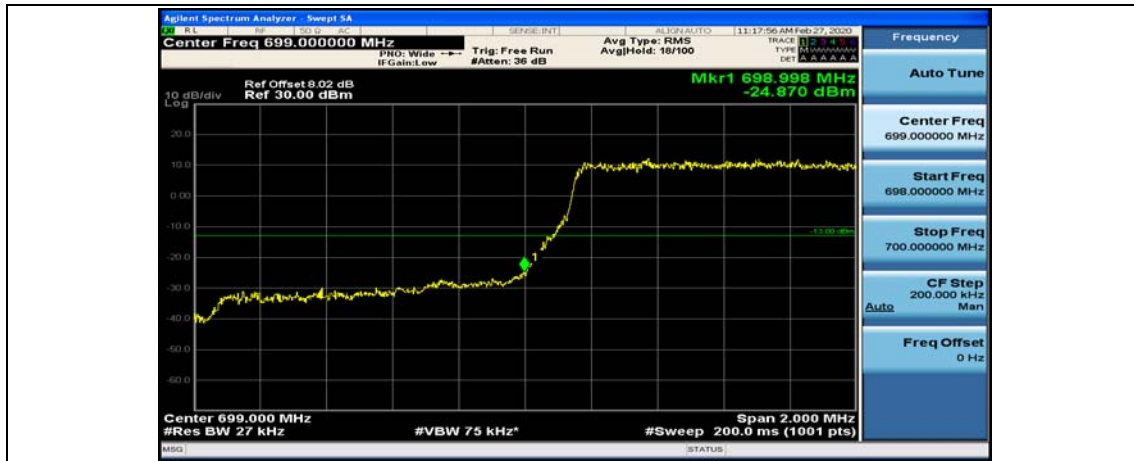
(Channel Bandwidth: 1.4 MHz)_HCH_QPSK_1RB#0
