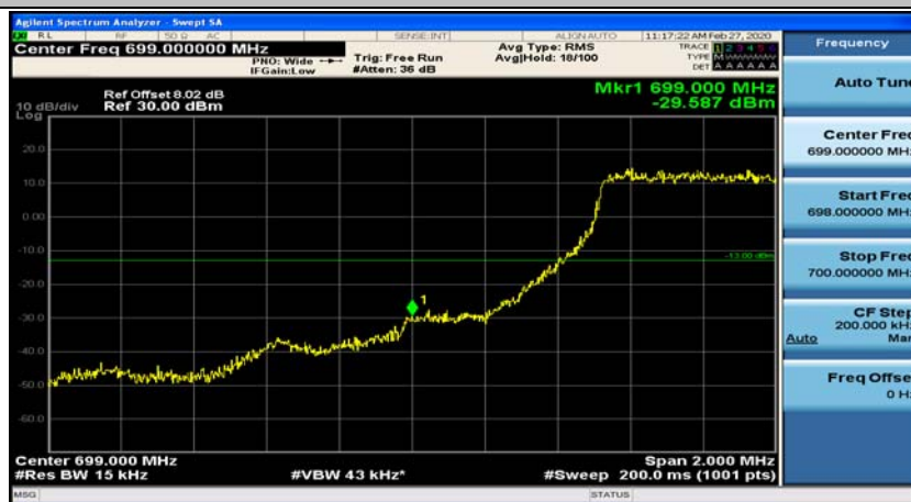
(Channel Bandwidth: 1.4 MHz)_LCH_QPSK_3RB#3
