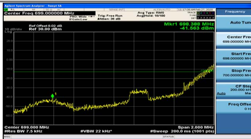
(Channel Bandwidth: 1.4 MHz)_LCH_16QAM_3RB#0
