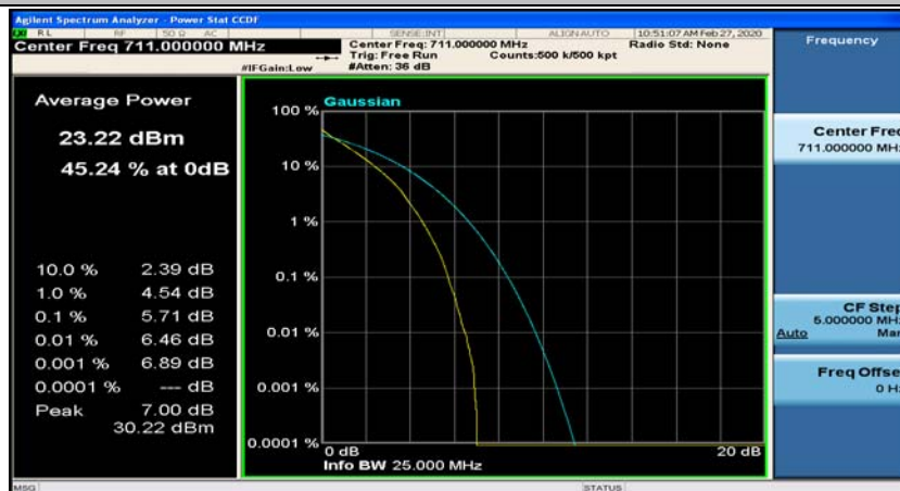
Channel Bandwidth: 10 MHz_HCH_QPSK_50RB#0
