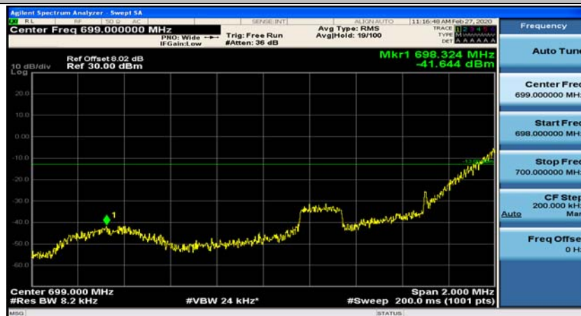
(Channel Bandwidth: 1.4 MHz)_LCH_QPSK_1RB#5
