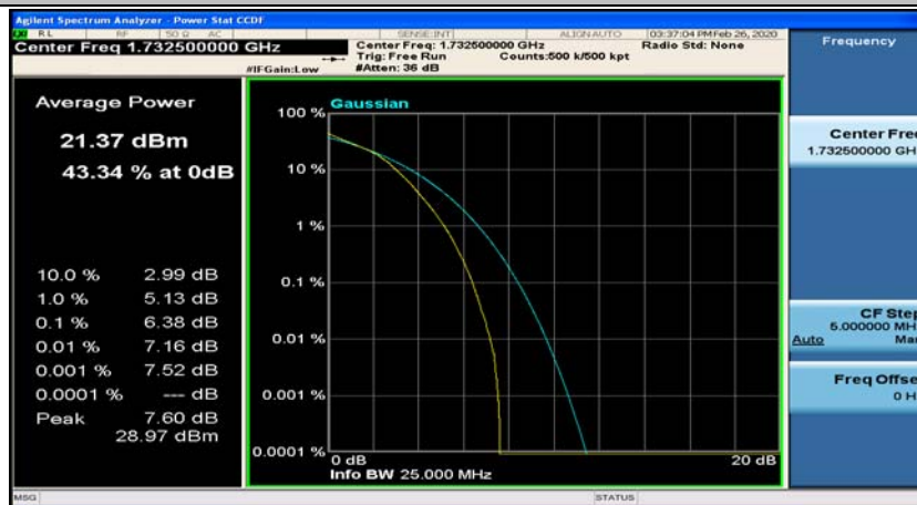
(Channel Bandwidth:20 MHz)_MCH_16QAM_100RB#0
