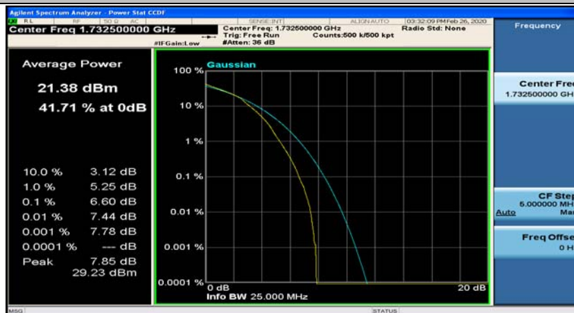
(Channel Bandwidth:15 MHz)_MCH_16QAM_37RB#18
