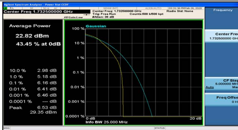
(Channel Bandwidth:15 MHz)_MCH_16QAM_1RB#74
