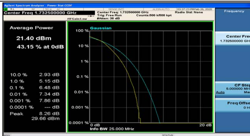
(Channel Bandwidth:20 MHz)_MCH_16QAM_100RB#0
