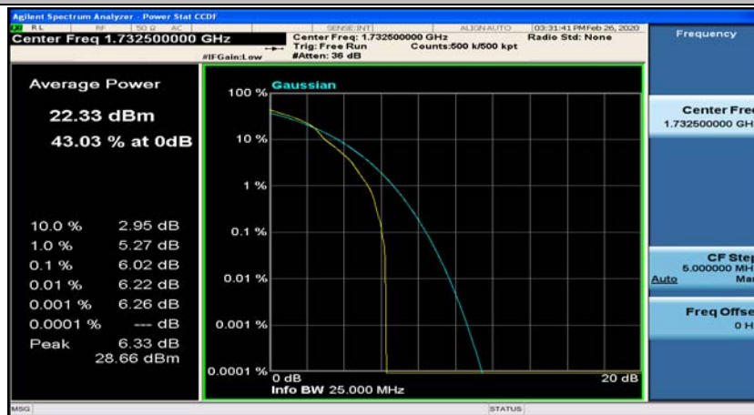
(Channel Bandwidth:15 MHz)_MCH_16QAM_37RB#0
