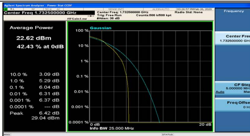
Channel Bandwidth: 10 MHz_MCH_16QAM_1RB#24
