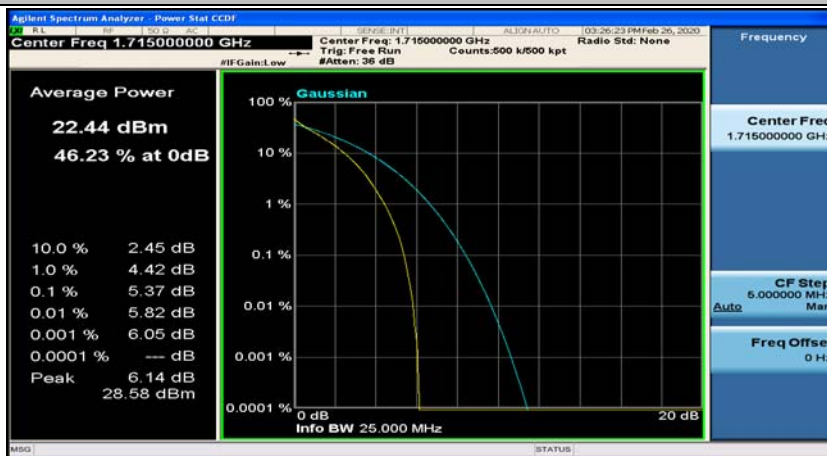
Channel Bandwidth: 10 MHz_LCH_QPSK_50RB#0
