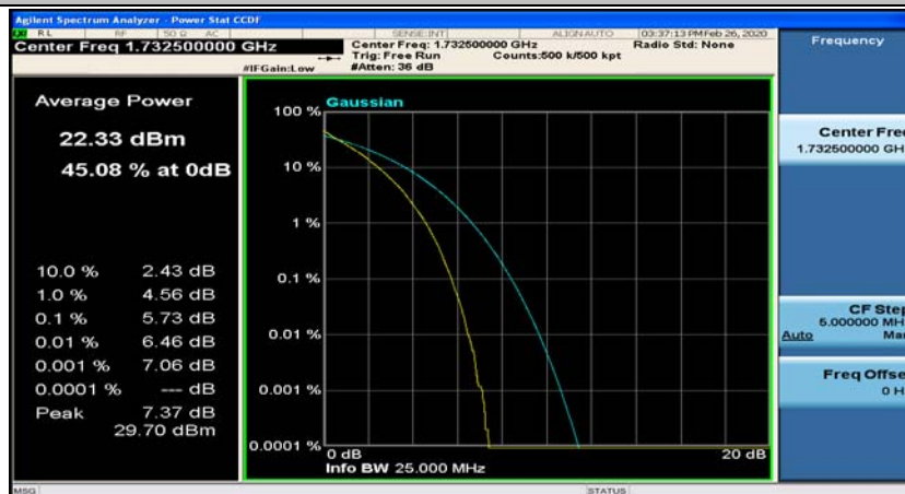
(Channel Bandwidth:20 MHz)_MCH_QPSK_100RB#0
