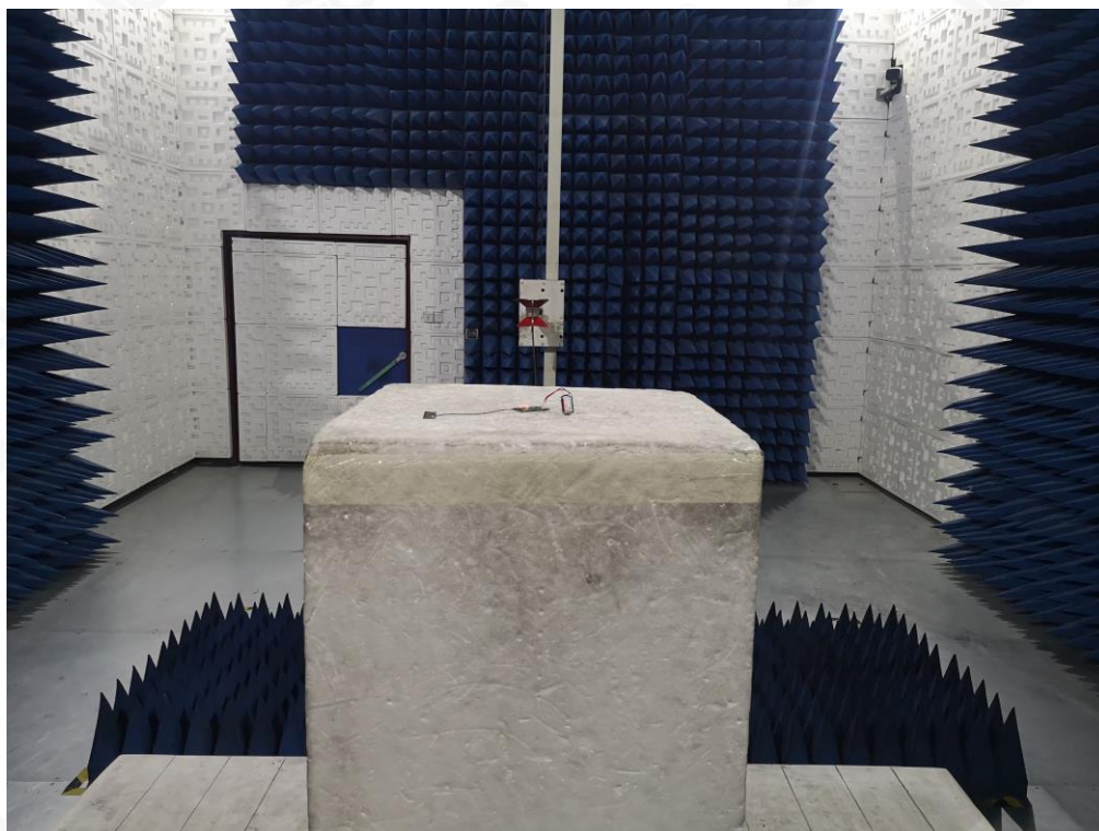
FCC RADIATED EMISSION TEST SETUP ABOVE 1GHZ
