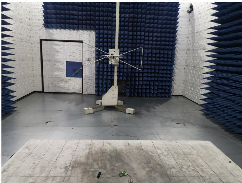
FCC RADIATED EMISSION TEST SETUP ABOVE 1GHZ
