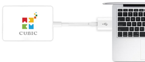
3.3-1 Cubic uses a serial cable to connect to the computer
