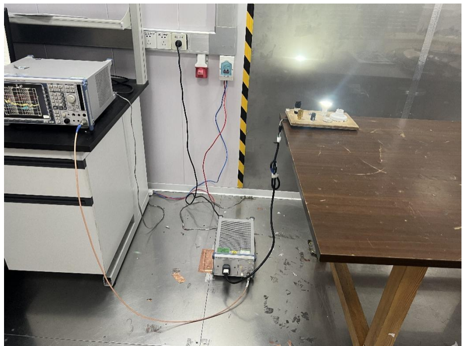
Conducted Emission Test Setup
