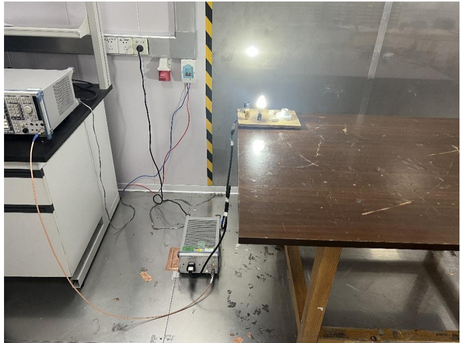
Conducted Emission Test Setup
