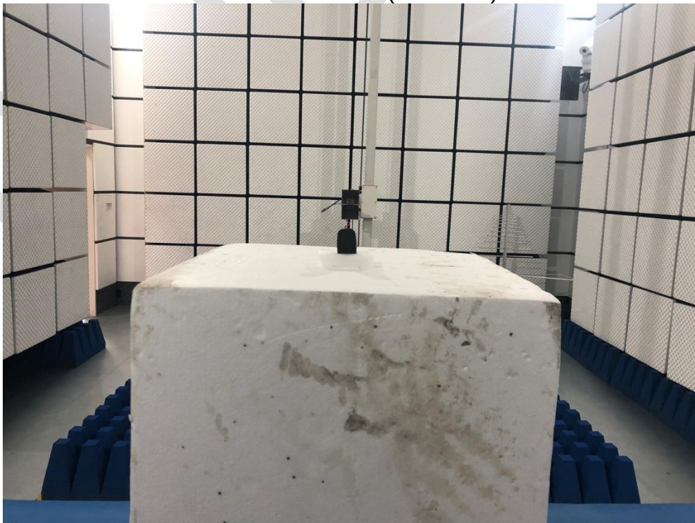
Radiated Emission(above 1G)
