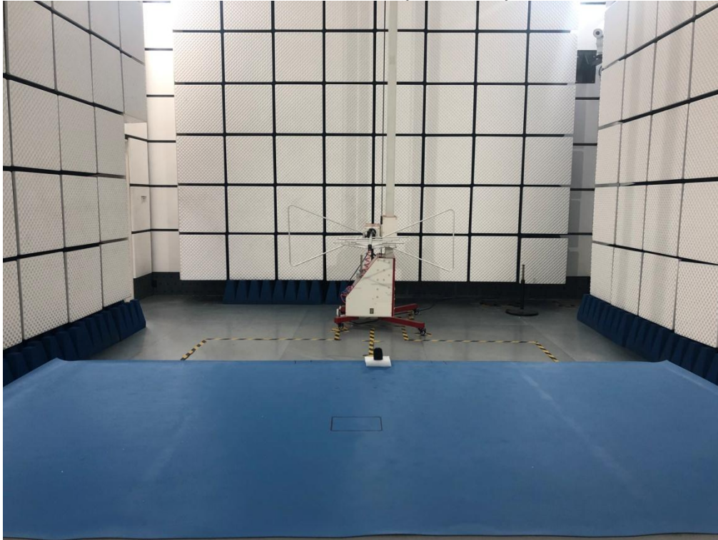
Radiated Emission(below 1G)
