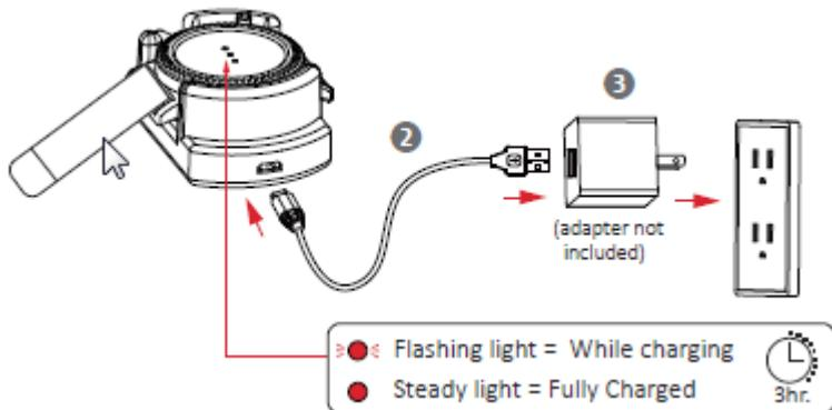
1. When the remote control charge reaches 30%, one of the LEDs will stop flashing (the other two LEDs flash alternately.)
