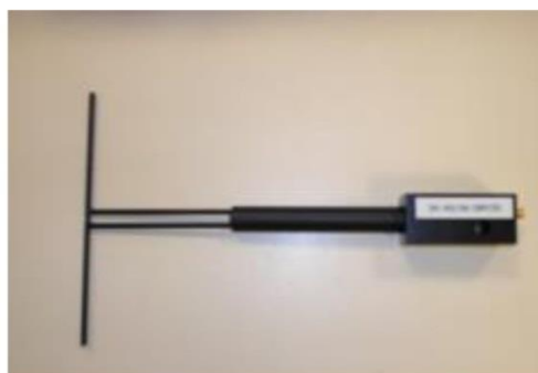
Figure 1 – Satimo COMOSAR Validation Dipole
