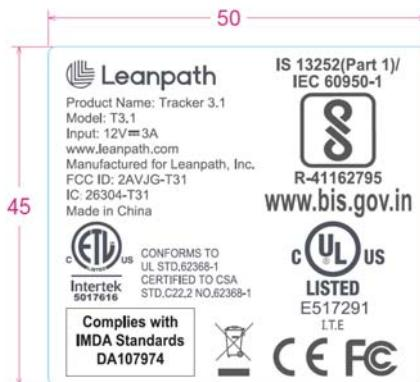
**Specifications:** The label shall be securely affixed to a permanently attached part of the device, in a location where it is visible or easily accessible to the user, and shall not be readily detachable. The label shall be sufficiently durable to remain fully legible and intact on the device in all normal conditions of use throughout the device's expected lifetime.
