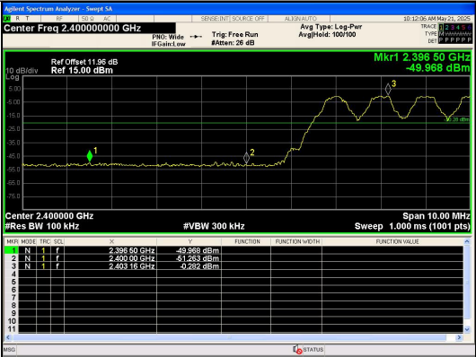
Out of Band Emission(Left) GFSK_DH5_Channel Hopping
