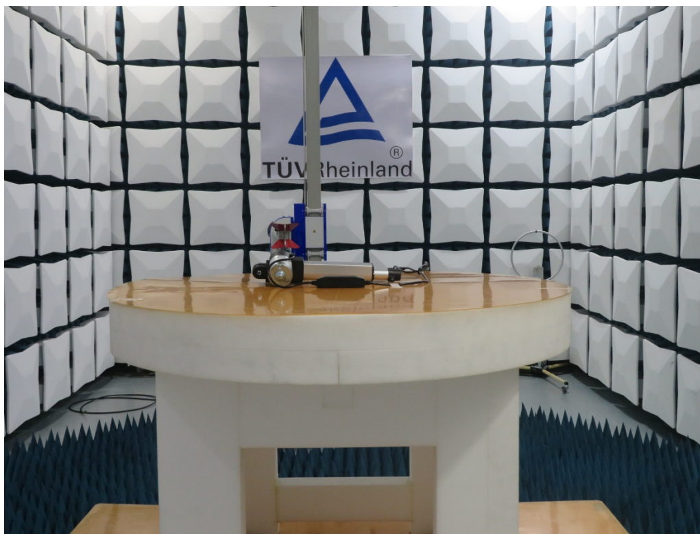
Photograph 3: Set-up photo for Radiated Emission, Above 1GHz
