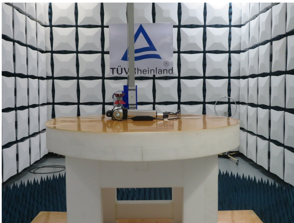
Photograph 3: Set-up photo for Radiated Emission, Above 1GHz
