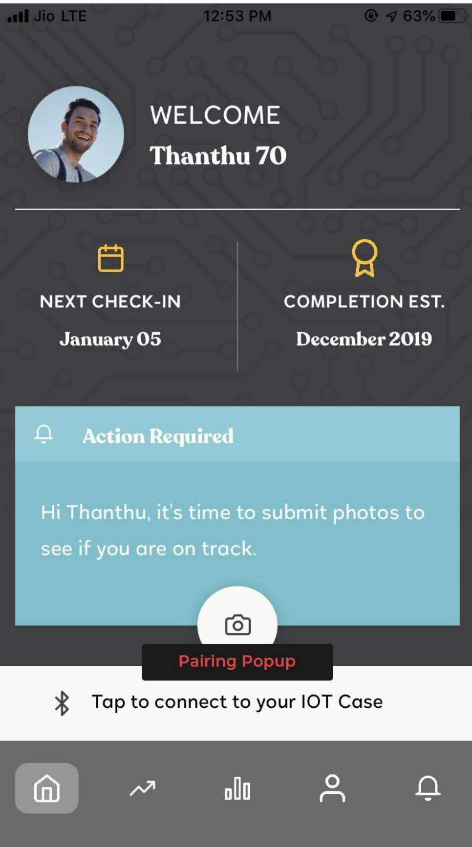
**3 Connecting to Bluetooth:** Tap the pairing button in the pairing popup screen. The app will show the toggle message once it connected successfully. The Bluetooth icon will appear on the app dashboard screen and IOTTrack screen when IOT is connected with the app.
