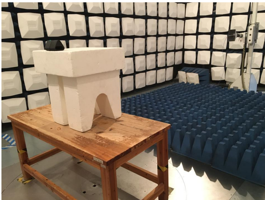
Test Setup For Radiated Emission (Above 1GHz)
