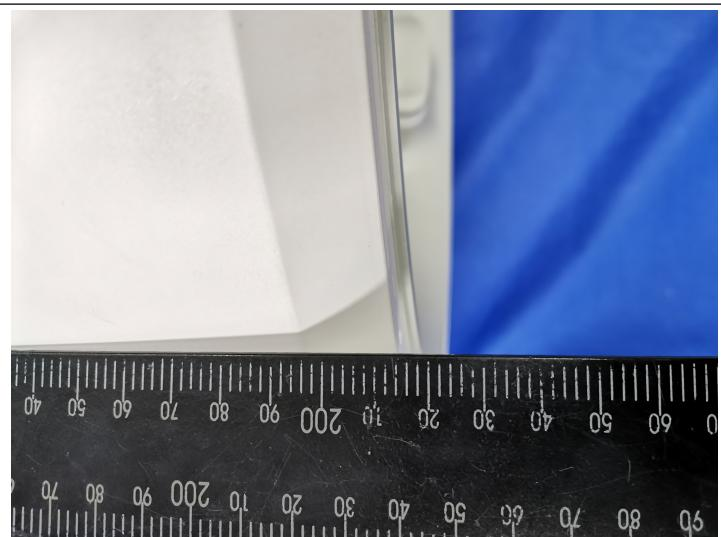
The distance between the edge of the antenna and the front of the device is 21.5cm, the width of the antenna is 1cm, and the actual effective distance is 20.5cm
