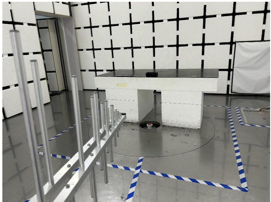
Radiation Emission Test Setup (30MHz to 1GHz)
