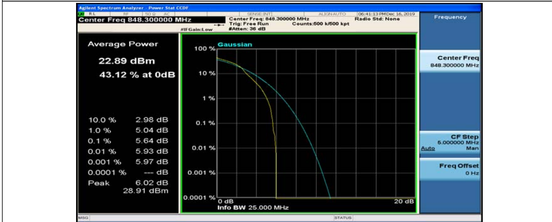
(Channel Bandwidth: 1.4 MHz)_HCH_16QAM_1RB#3
