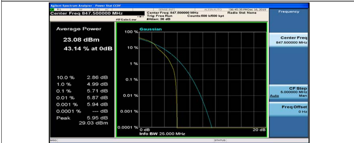
(Channel Bandwidth: 3 MHz)_HCH_16QAM_1RB#7
