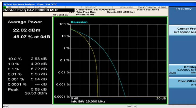
(Channel Bandwidth: 3 MHz)_HCH_QPSK_15RB#0
