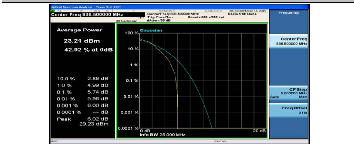
(Channel Bandwidth: 5 MHz)_MCH_16QAM_1RB#12
