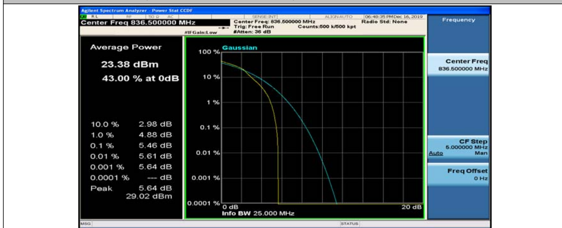
(Channel Bandwidth: 5 MHz)_MCH_16QAM_1RB#24
