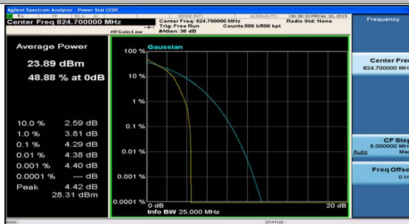
(Channel Bandwidth: 1.4 MHz)_LCH_QPSK_3RB#0
