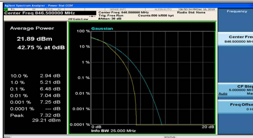
(Channel Bandwidth: 5 MHz)_HCH_16QAM_12RB#6
