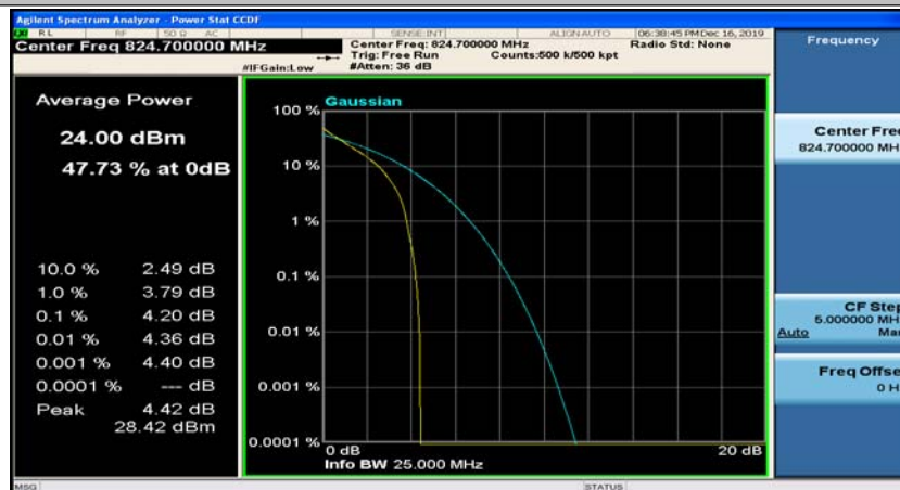
(Channel Bandwidth: 1.4 MHz)_LCH_QPSK_6RB#0
