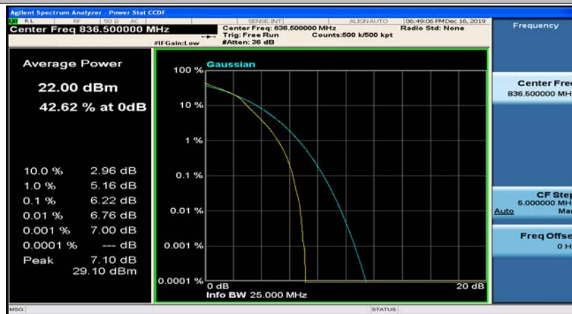
(Channel Bandwidth: 5 MHz)_MCH_16QAM_12RB#6
