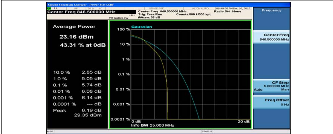
(Channel Bandwidth: 5 MHz)_HCH_16QAM_1RB#12
