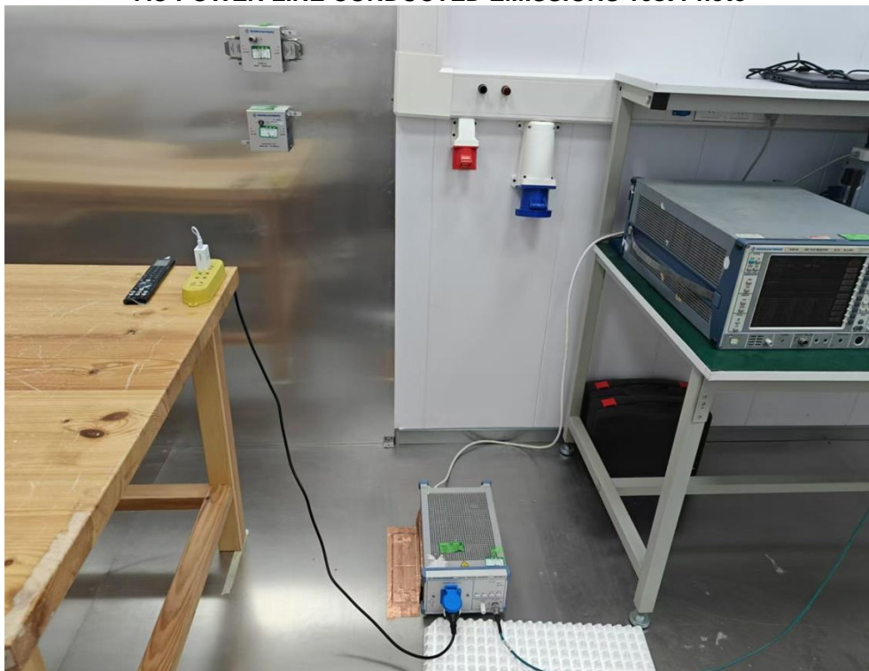
AC POWER LINE CONDUCTED EMISSIONS Test Photo
