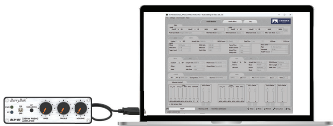
Figure 1: Connect the BLV-D1 to a personal computer or laptop and ensure that you have installed the ACP Workbench application.
