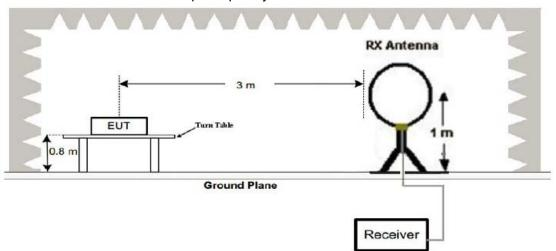
(2) Radiated Emission Test-Up Frequency 30MHz~1GHz
