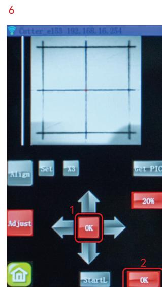
Press and hold the OK button until all the four direction buttons turn red. Then click the OK button and the machine will start to draw four squares for calibration.
