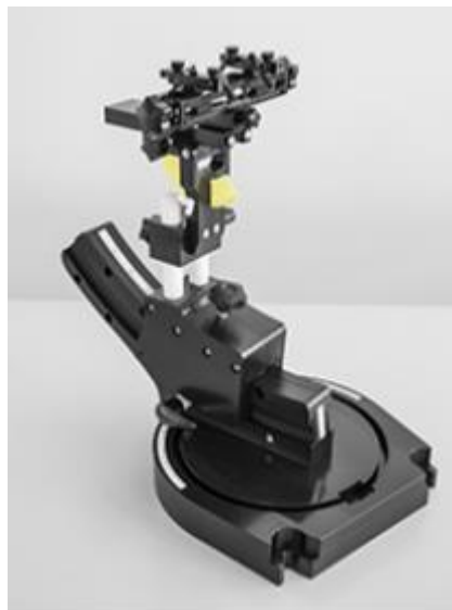
Device holder supplied by SPEAG
