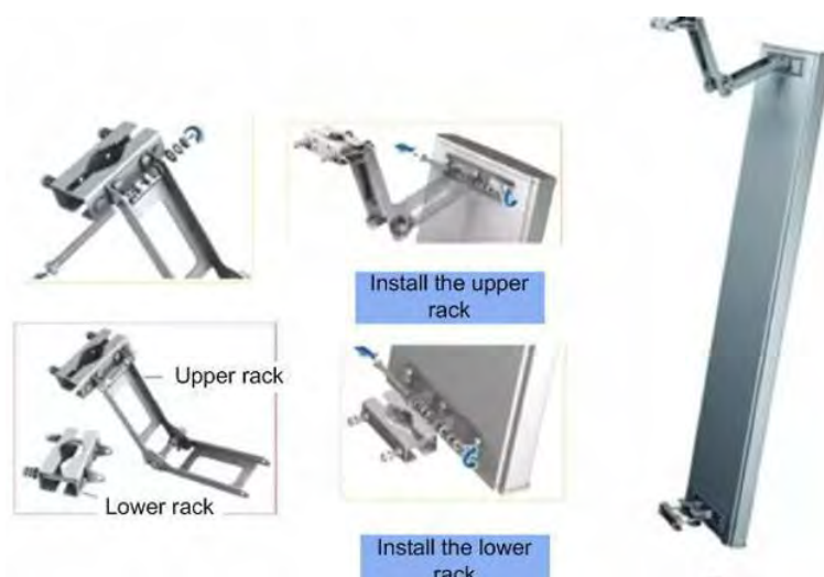
Figure 3-11 Installer Assembling Procedure of Directional Antennas
