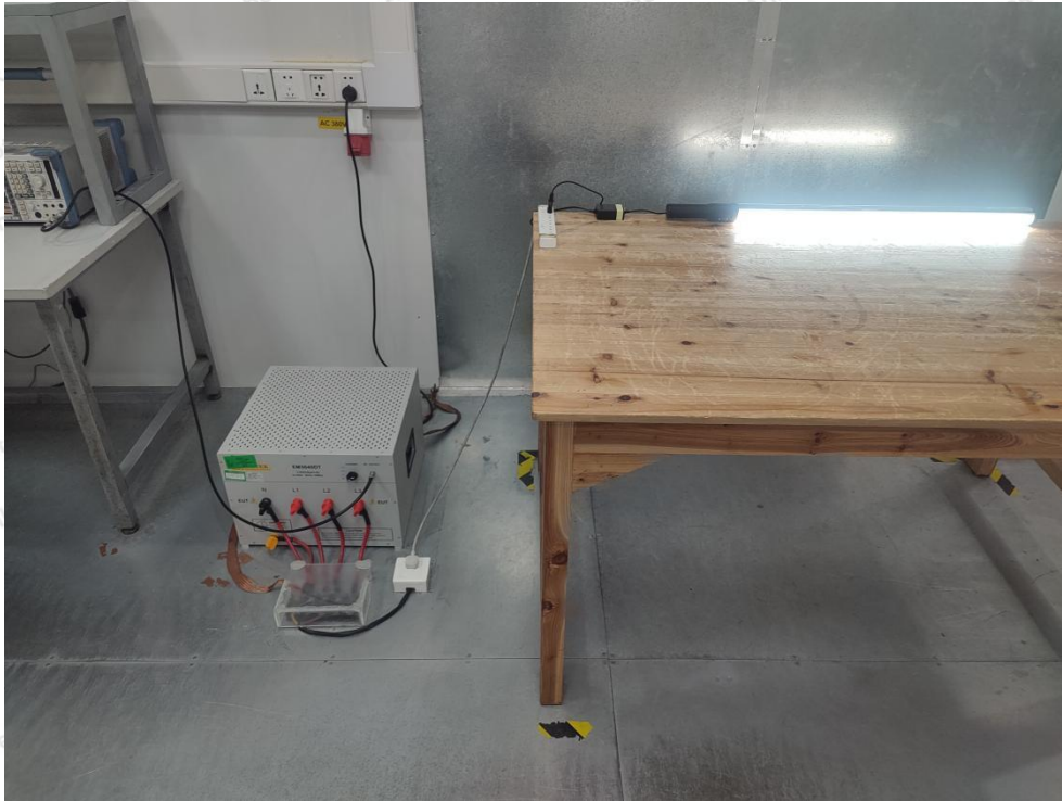
Photo of Conducted Emission Measurement
