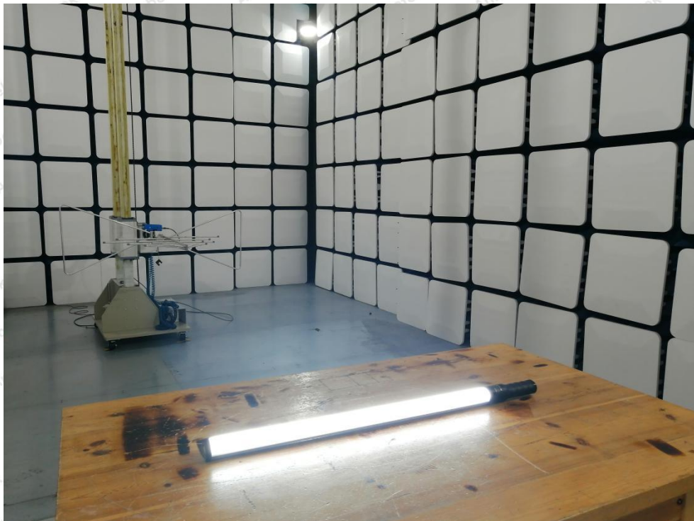
Photo of Radiation Emission Test
