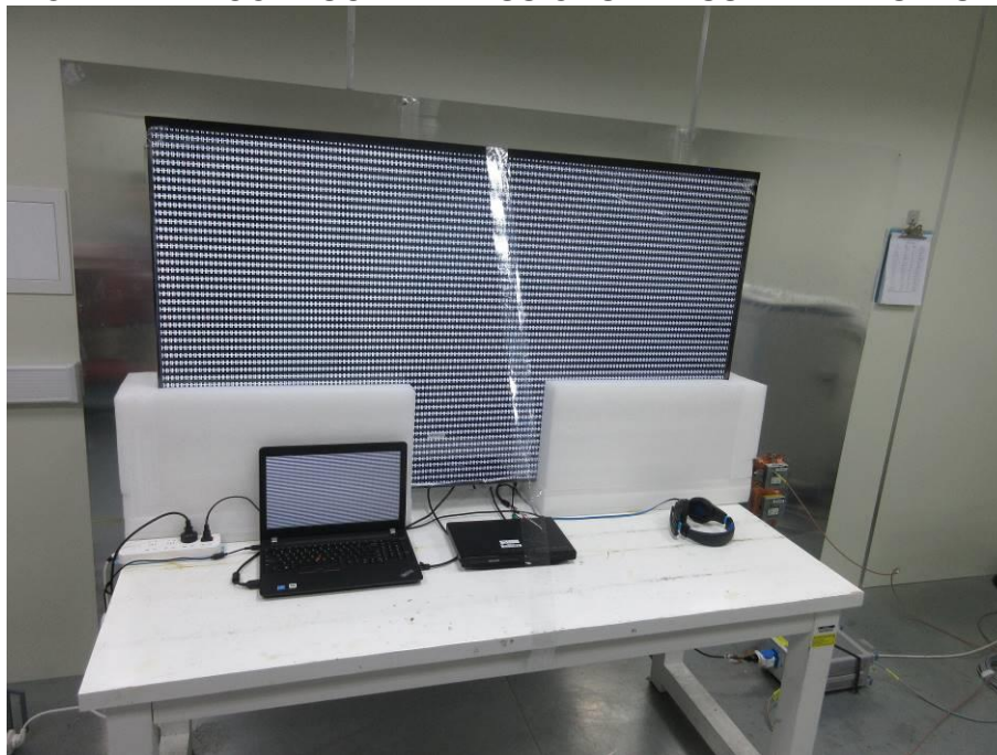
POWERLINE CONDUCTED EMISSIONS MEASUREMENT SETUP
