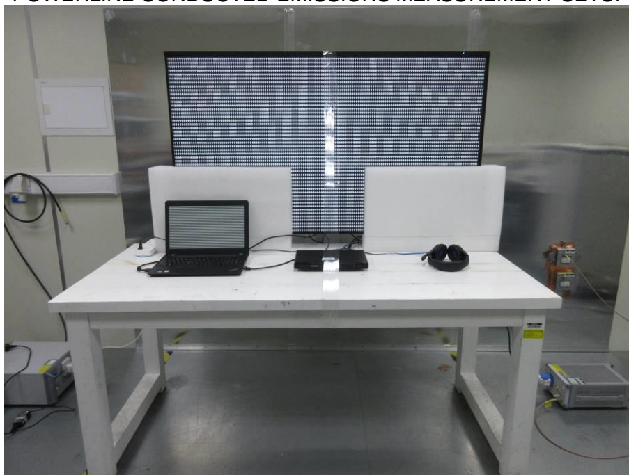
POWERLINE CONDUCTED EMISSIONS MEASUREMENT SETUP
