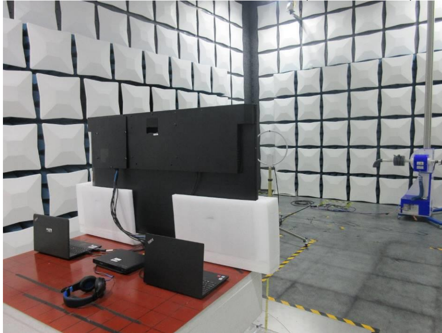
RADIATED RF MEASUREMENT SETUP (9KHz ~ 30 MHz)
