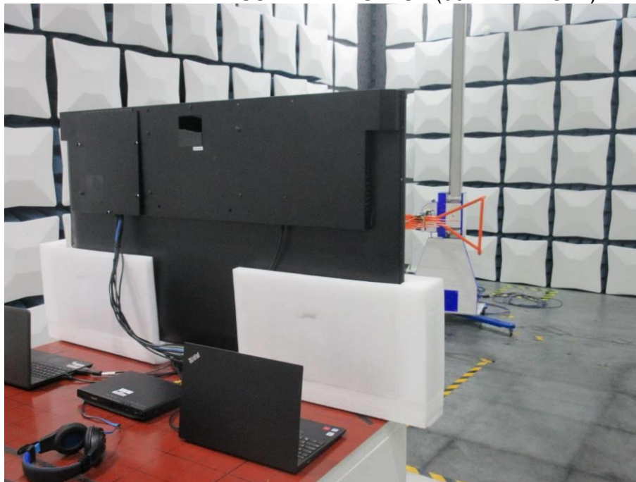
RADIATED RF MEASUREMENT SETUP (30MHz ~ 1 GHz)
