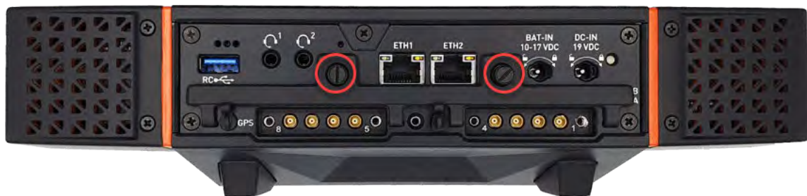
SIM flap screw location
