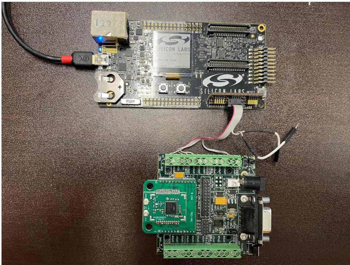
**Simplicity Commander** from Silicon Labs is used to flash the firmware onto the module.
