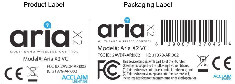
Specifications: The label shall be securely affixed to a permanently attached part of the device, in a location where it is visible or easily accessible to the user, and shall not be readily detachable. The label shall be sufficiently durable to remain fully legible and intact on the device in all normal conditions of use throughout the device's expected lifetime.
