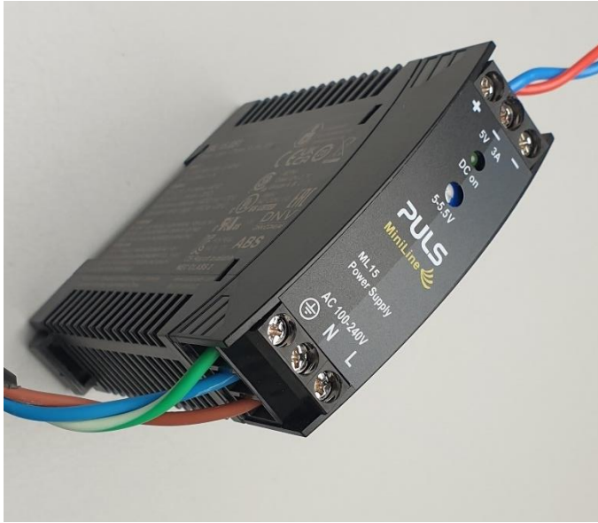
Photo 6. AC/DC power supply.
