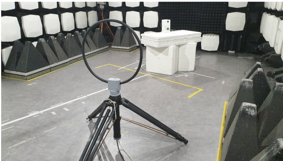
Photo 11. Radiated emission test setup in SAC. 9 kHz – 30 MHz.
