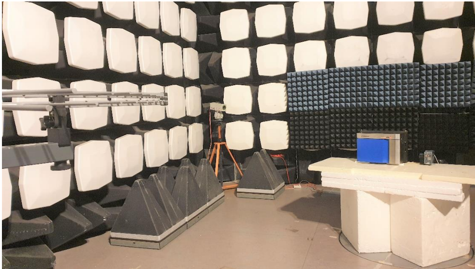
Photo 8. Radiated emission test setup in SAC. 200 - 1000 MHz.
