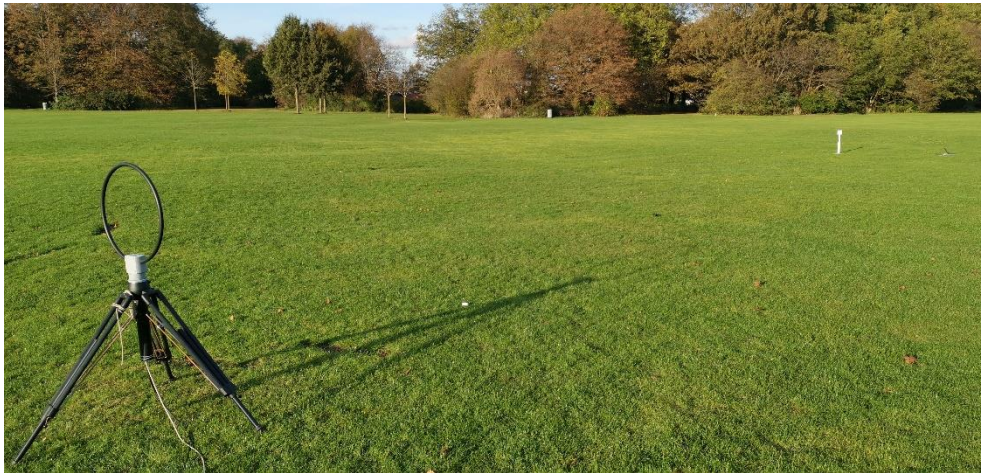
Photo 5. Radiated emission test setup at OATS. 9 kHz – 30 MHz
