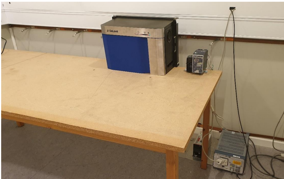
Photo 9. AC Conducted emission test set up.
