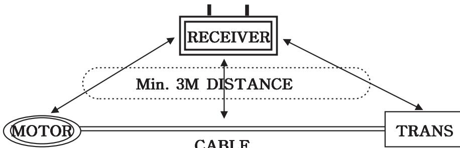
9. Install receiver top outside of electrical control box and installation in inside the control box is not a proper method.
