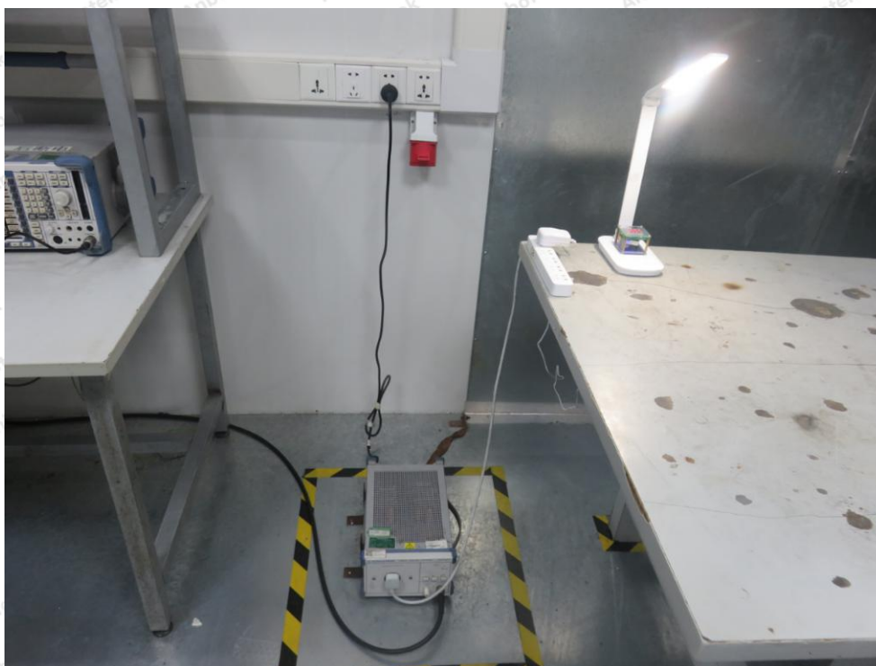
Photo of Conducted Emission Measurement
