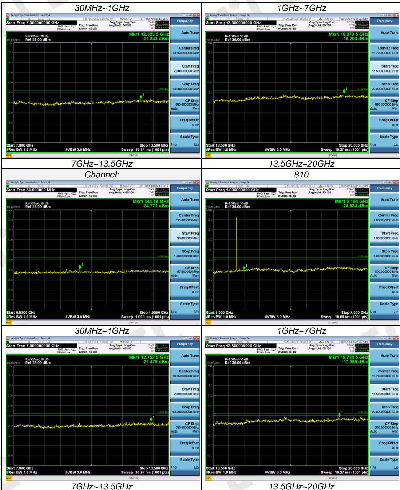
**Radiated Measurement:****GSM 850**
