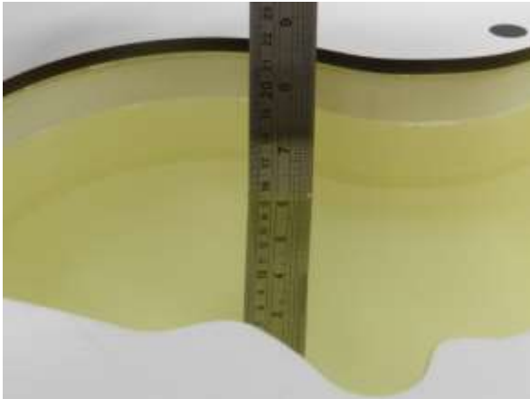
Fig 11.1 Photo of Liquid Height for Head SAR
