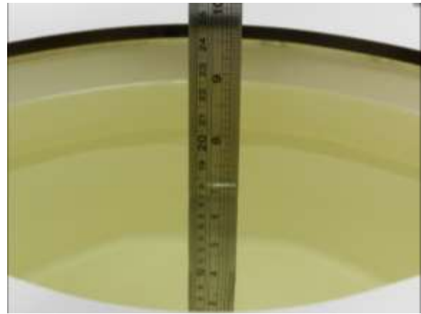
Fig 11.2 Photo of Liquid Height for Body SAR
