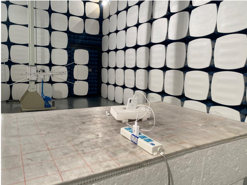
Radiated Spurious Emission Below 1GHz
