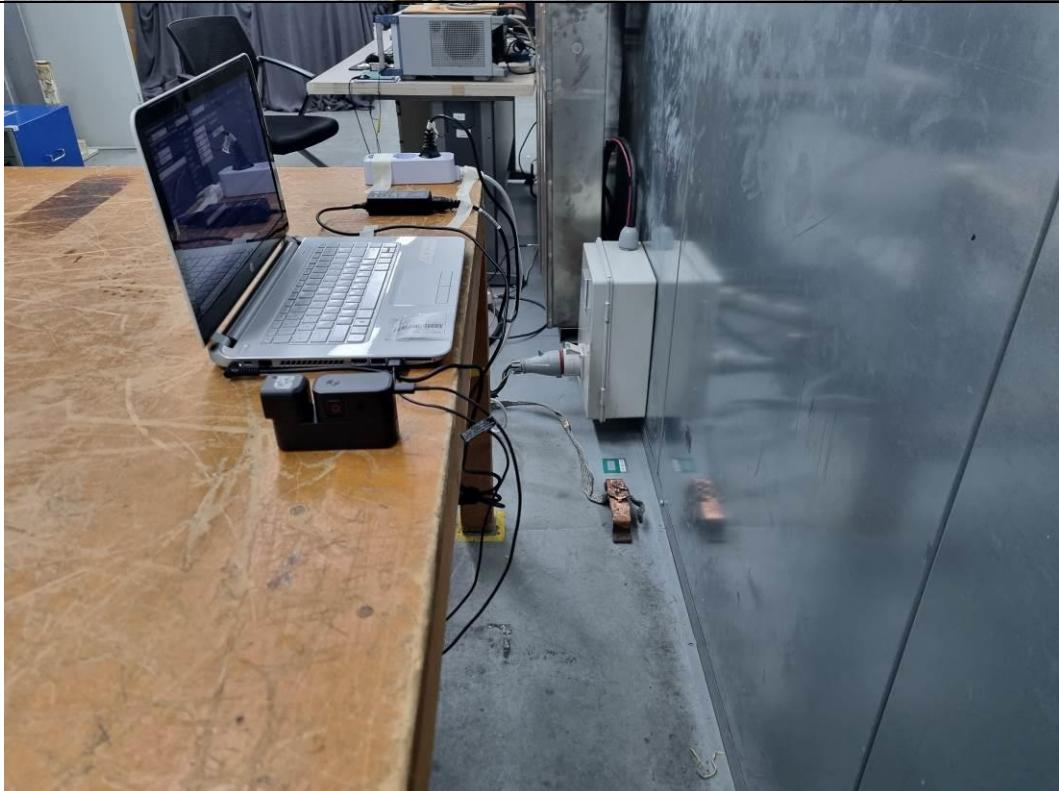
**- Radiated Emission Test (Below 1 GHz)**
